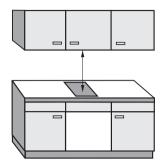
When two or more appliances are installed together below a cooker hood, e.g. a grill and an induction hob combiset, which have different safety distances given in the installation instructions, you should select the greater distance of the two.
